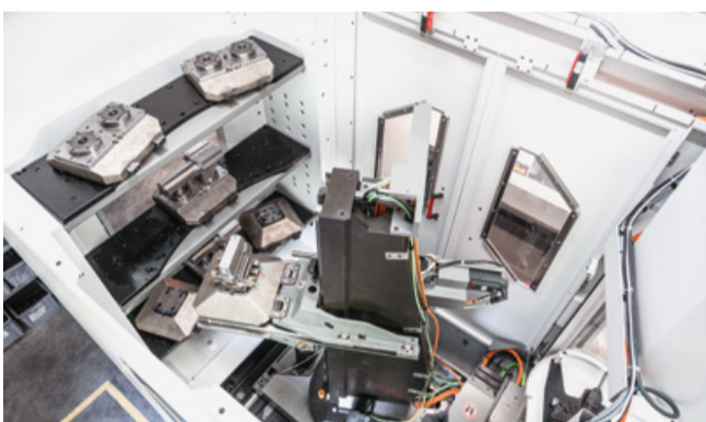
Since Wiegemann also mills smaller products, some of which only run for 10 or 20 minutes, the mould maker this time opted for an automated machining centre: The C 42 U with HS flex.
