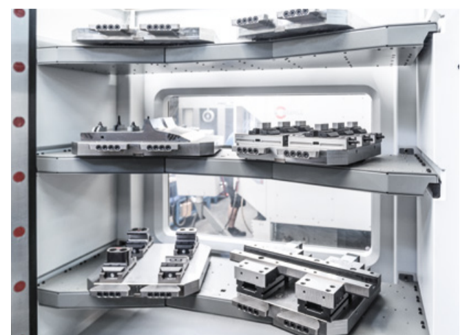
Cafmeyer also utilises the C 650 U for smaller components – and places them together on one pallet for efficient machining.
