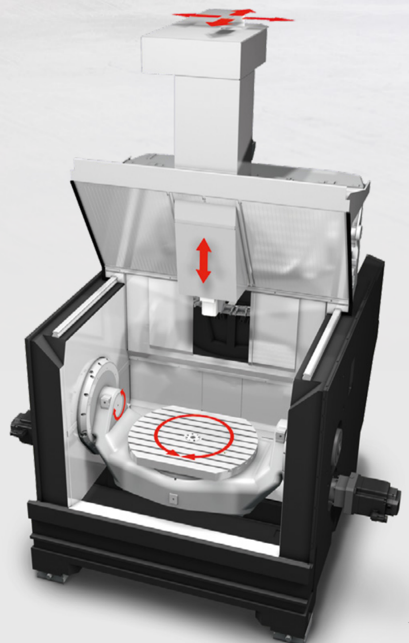
Efficient milling operations with 5-axis technology: Three axes in the tool, two axes in the workpiece.
