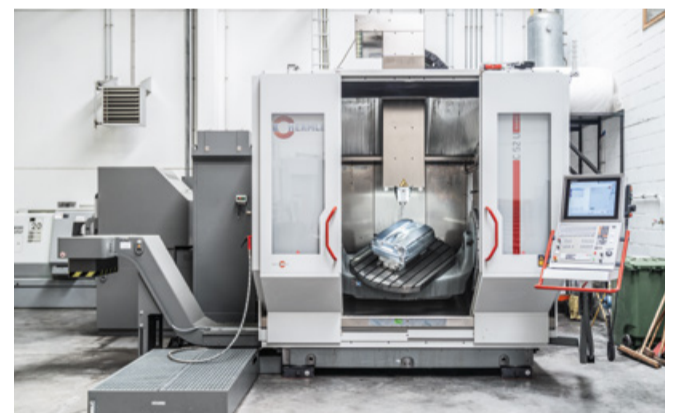
With its working range of 1,000 x 1,100 x 750 millimetres and a vertical table clearance of 950 millimetres, the C 52 U offers space even for the largest of moulds.
