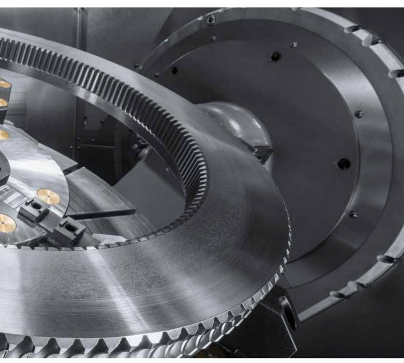
Machine construction. Gearwheel with worm gear external splines and straight internal splines produced by hob peeling.
