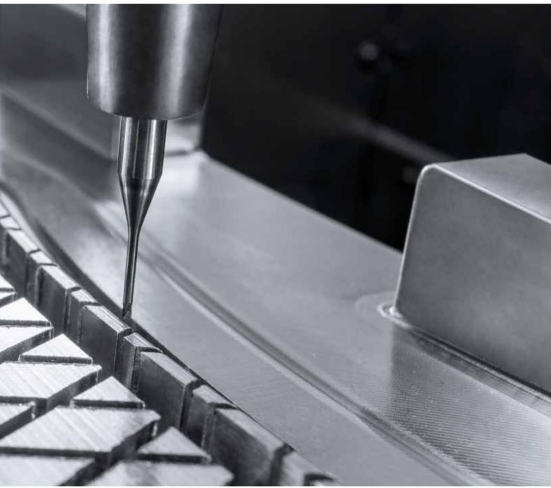
Tool and mold making. Rib component made of tool steel for a shoe sole die mold. 5-axis simultaneous machining using a sophisticated groove cutting strategy.
