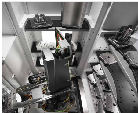
HS flex with two pallet storage modules and a setup station, adapted to a C 42 machining centre.
