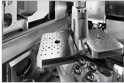
Double gripper for 2 x 150 kg
